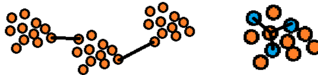
Fig. 9. Illustration for coordination numbers intra-phase CNHH (left), and inter-phase CNHE (right)
